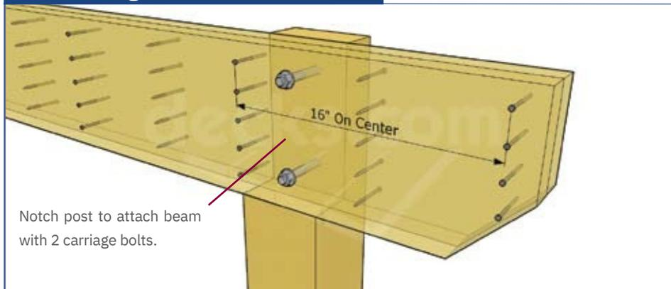
Notch post to attach beam with 2 carriage bolts.
