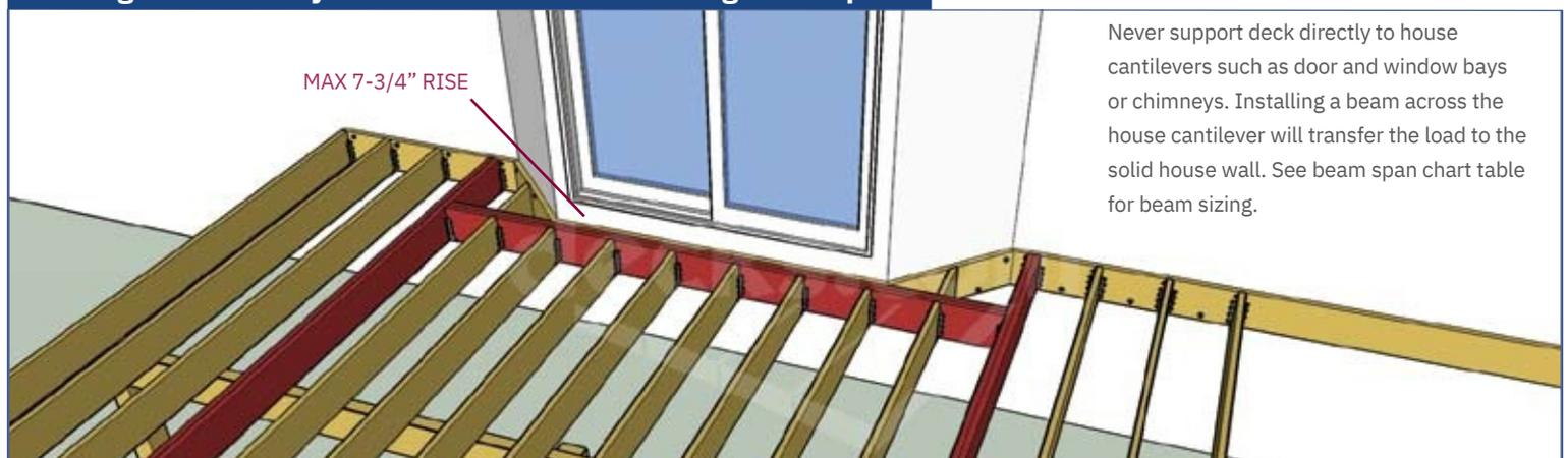
Never support deck directly to house cantilevers such as door and window bays or chimneys. Installing a beam across the house cantilever will transfer the load to the solid house wall. See beam span chart table for beam sizing.
