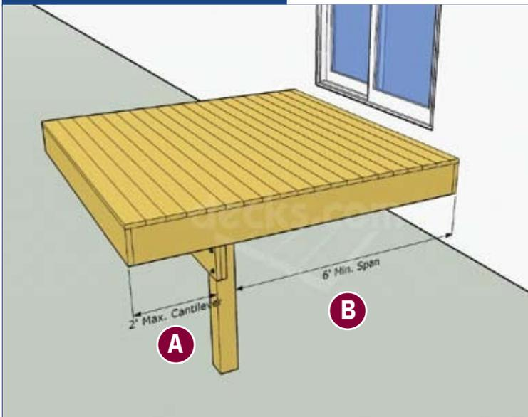
2' maximum cantilever - 6' minimum joist span for cantilever decks.
